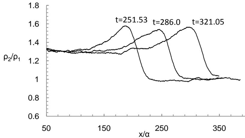
Figure 2: The average density profile related to the distance from the piston for  $Q/e_1=25$  at three different time steps
