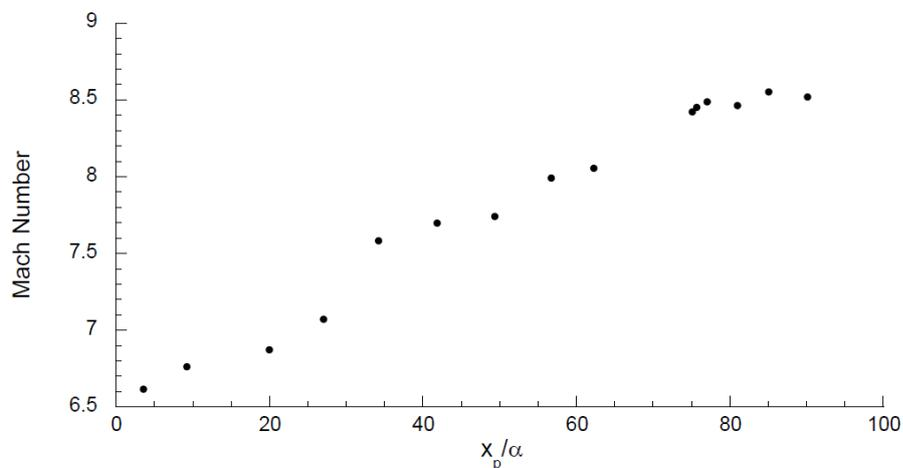
Figure 4: Evolution of the Mach number of the reaction and shock front propagating through the medium, compared to the piston location, with  $Q/e_I=25$  and  $u_p^2/e_I=8$
