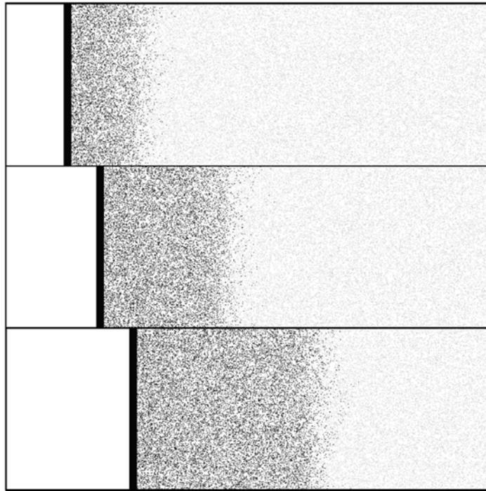
Figure 3: Snapshots of the reaction and shock wave progressing through the reactive hard disk medium, with  $Q/e_I=25$  and  $u_p^2/e_I=8$ (Note: The size of the disks was amplified four times to better see their locations)
