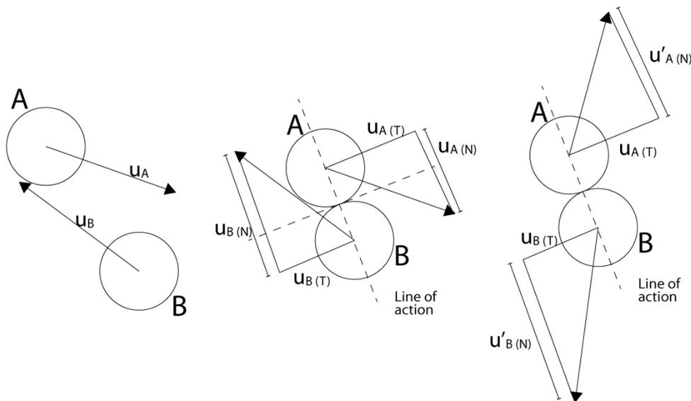
Figure 1: Kinematics of collision between particles A and B before impact(left), during impact(center) and immediately after collision(right)
