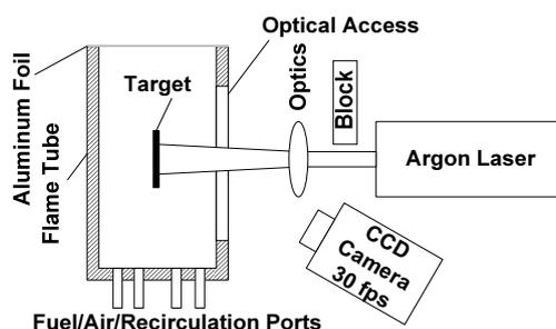
Figure 1: Diagram of flame tube configuration.
