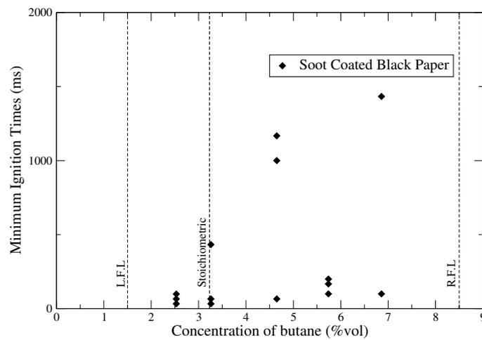
Figure 4: Time to ignition for soot coated black paper for different mixture composition (flux = 5.5 MW/m<sup>2</sup>). Longer ignition times are attributed to variations in the soot coating.
