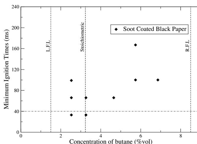
Figure 5: Time to ignition for soot coated black paper for different mixture composition (flux =  $5.5 \text{ MW/m}^2$ ). Ignition times lower than 100 ms were found plausible across all equivalence ratios while ignition times reduced under 40 ms in stoichiometric and leaner mixtures.
