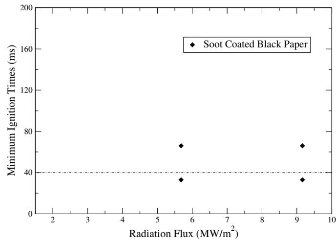
Figure 3: Time to ignition for soot coated black paper in a butane/air mixture ( $\phi = 1.0$ ). Ignition times below 40 ms could be observed.
