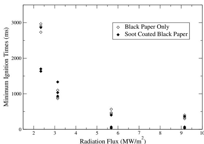
Figure 2: Time to ignition for black paper in a butane/air mixture ( $\phi = 1.0$ ). Shorter ignition time can be seen for higher levels of radiation flux. Longer ignition times are attributed to variations in the soot coating.
