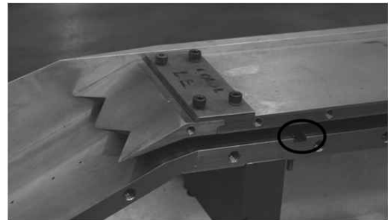
Figure 2. W-shape cowl and cavity flame holder
