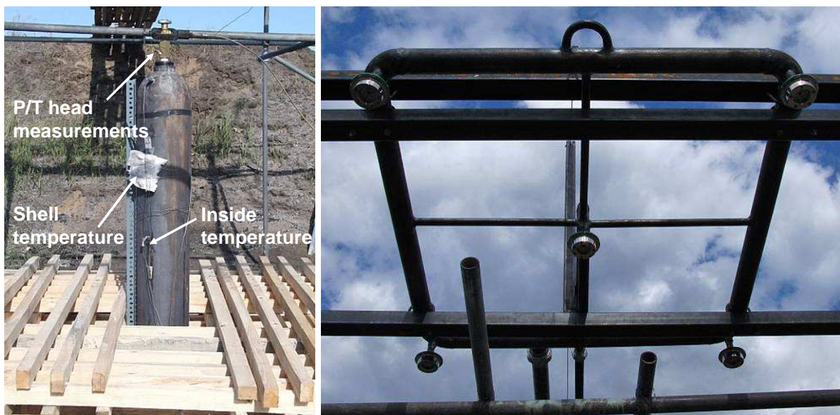
Figure 1. Acetylene cylinder prepared for the bonfire test (left) and detail of the cooling system (right).
