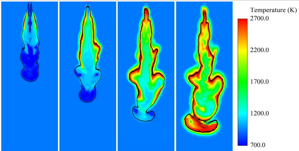
Figure 3: Temperature evolution for time  $t = 300\mu s$ ,  $t = 400\mu s$ ,  $t = 500\mu s$  et  $t = 600\mu s$ . The black line represents the stoichiometric mixture fraction
