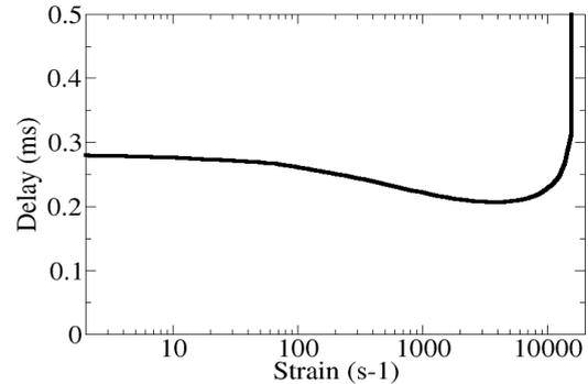
Figure 5: simulation of a 1D flamelet auto-ignition delay at the stoichiometric mixture fraction showing strain limit value of  $17.000 s^{-1}$ .
