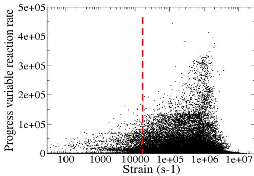
Figure 4: Scatter plot of  $\tilde{\omega}_c$  as a function of the strain at  $t = 300\mu s$  (just after start of auto-ignition). The red line represents the limit of auto-ignition as shown in fig. 5
