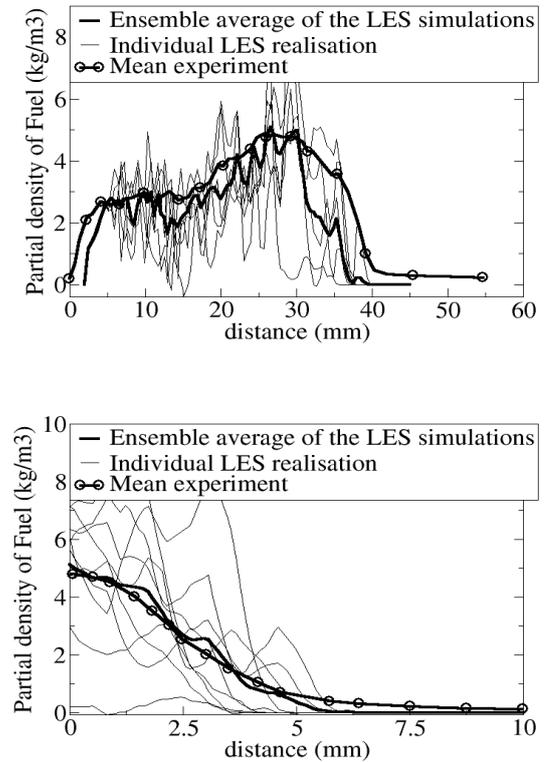
Figure 2: Comparison of the fuel partial density along the injector axis (top) and along a radial profile (bottom) located 30 mm downstream of the injector at  $t = 500\mu s$
