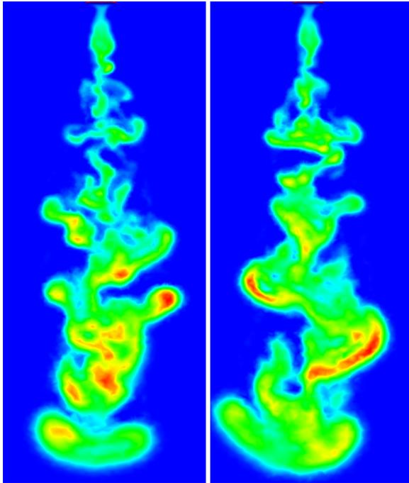
Figure 1: Snapshots of the partial fuel density at  $t = 500\mu s$  for two different realisations (i.e. different initial turbulence)
