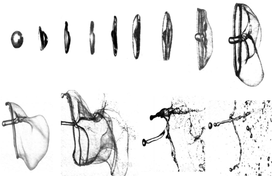
Figure 1. Water droplet break-up mechanism (type inverted bag-jet break up). Measured in 30 cm x 30 cm cross-section wind tunnel. Initial droplet size 4.2 mm. Steady flow of 15 m/s. [34].
