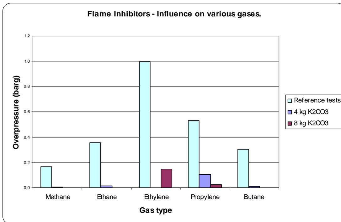
Figure 2. Peak explosion pressure in the 50 m<sup>3</sup> module for a series of hydrocarbon fuels using potassium carbonate as an inhibitor. The quantity of inhibitor was varied and ignition was effected 2 s after inhibitor injection.
