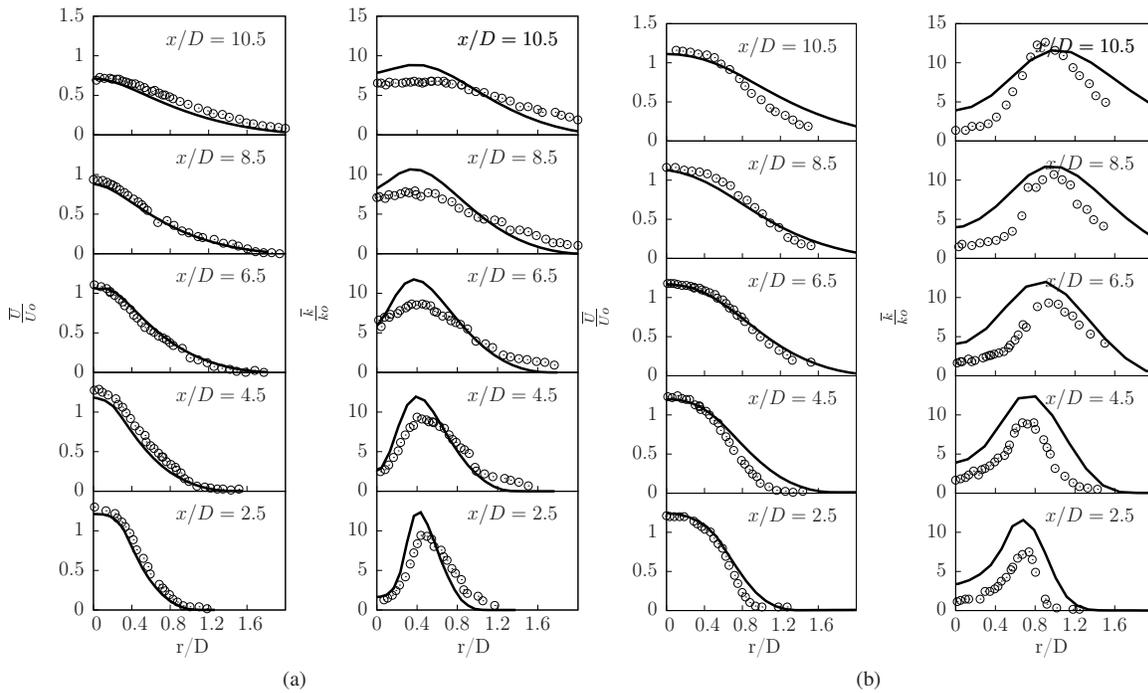
Figure 2: The calculated (lines) normalised mean axial velocity and turbulent kinetic energy from (a) non-reacting and (b) reacting flows are compared to the the measurements (symbols).
