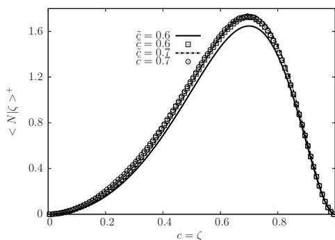
Figure 1: Comparison of modelled, Eq. (2) (lines), conditional mean scalar dissipation rate and DNS (symbols) results. The values are non-dimensionalised using  $S_L^o$  and  $\delta_L^o$ .
