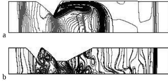
Fig.2 Isopicts (grey) and level lines of density of reactive component (black) of flows in channels with one (a) and two (b) constrictions.
