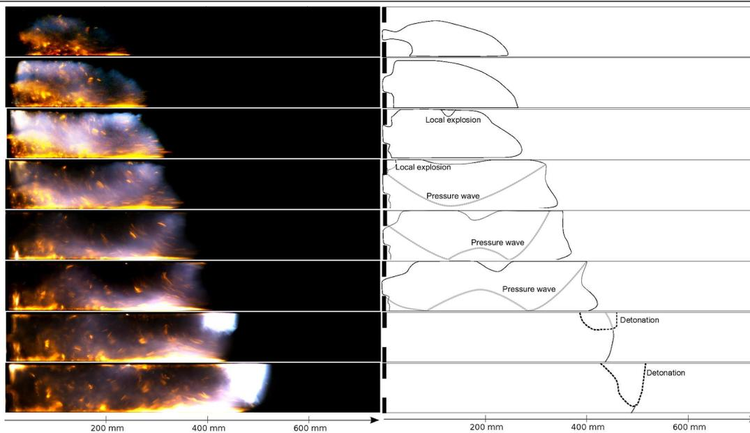
Figure 3: Photos and sketch of the flame propagation and development of detonation. Time difference between frames are  $1/30000\text{sec}$ .  $30\% H_2$  in air with  $BR = 0.84$ .
