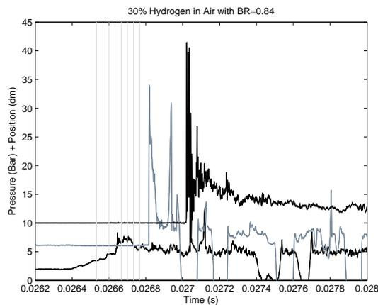
Figure 4: Pressure record of experiment. 30%  $H_2$  in air with  $BR = 0.84$ . The vertical lines correspond to the frames of figure 3.
