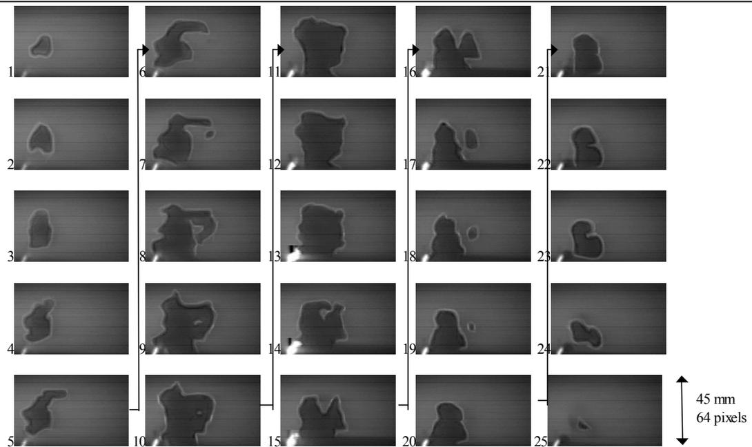
Figure 2. Twenty five “slices” through a methane-air flame at “one instant”,  $\phi=0.6$ ,  $u_f=0.09$  m/s,  $u' = 0.56$  m/s and 28.9 ms from ignition. Separation of 0.7 mm between the images.
