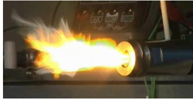
Figure 3. The lab scale hybrid rocket fuel grain could be ignited successfully by N_2O catalytic decomposition gas (without nozzle).
