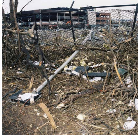
Figure 5: Fuji carpark lampposts: Lamppost in foreground has been hit by blast, snapped and then felled NE. The Fuji carpark Buncefield perimeter fence has next been blown down, up over the felled lamppost base, and then dragged over the fallen pole. A similar pole in the background has also been snapped and blown down to the E.
