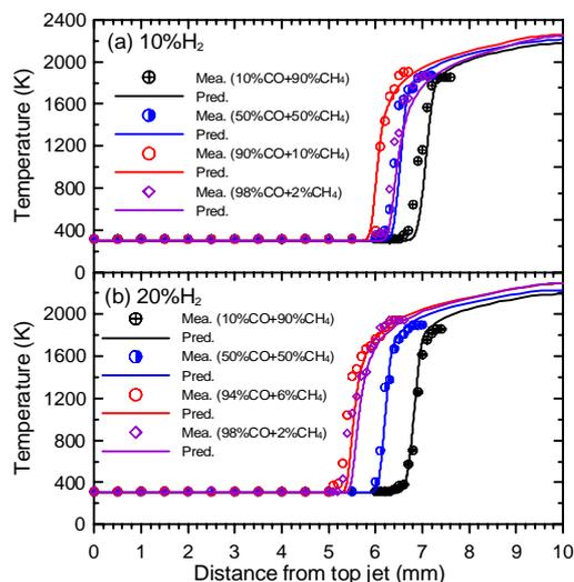
Fig. 4. Comparison of the measured and calculated flame temperatures for the premixed stoichiometric H<sub>2</sub>/CO/CH<sub>4</sub>/air flames: (a) 10% H<sub>2</sub> and (b) 20% H<sub>2</sub>.
