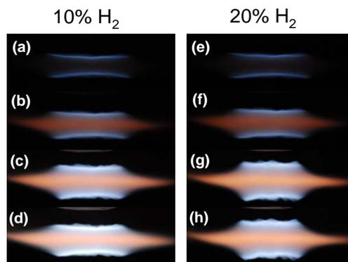
Fig. 3. Photographs of the premixed opposed-jet flames. (a): flame #1, (b): #2, (c): #3, (d): #4,; (e): #5, (f): #6, (g): #7, (h): #8.
