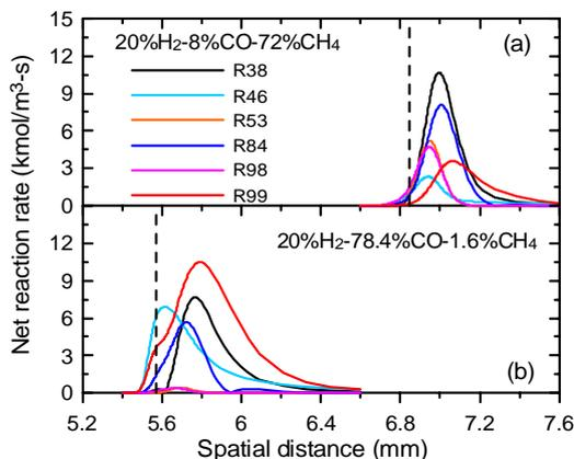
Fig. 5. Computed axial distributions of net reaction rate for flames 5 and 8.
