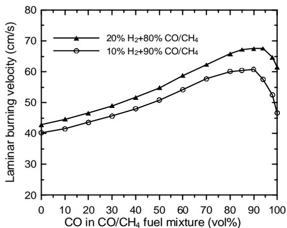
Fig. 2. Computed laminar burning velocity of the stoichiometric H<sub>2</sub>/CO/CH<sub>4</sub>/air flames as a function of CO contents in the CO/CH<sub>4</sub> fuel mixture with 10% and 20% H<sub>2</sub> additions.
