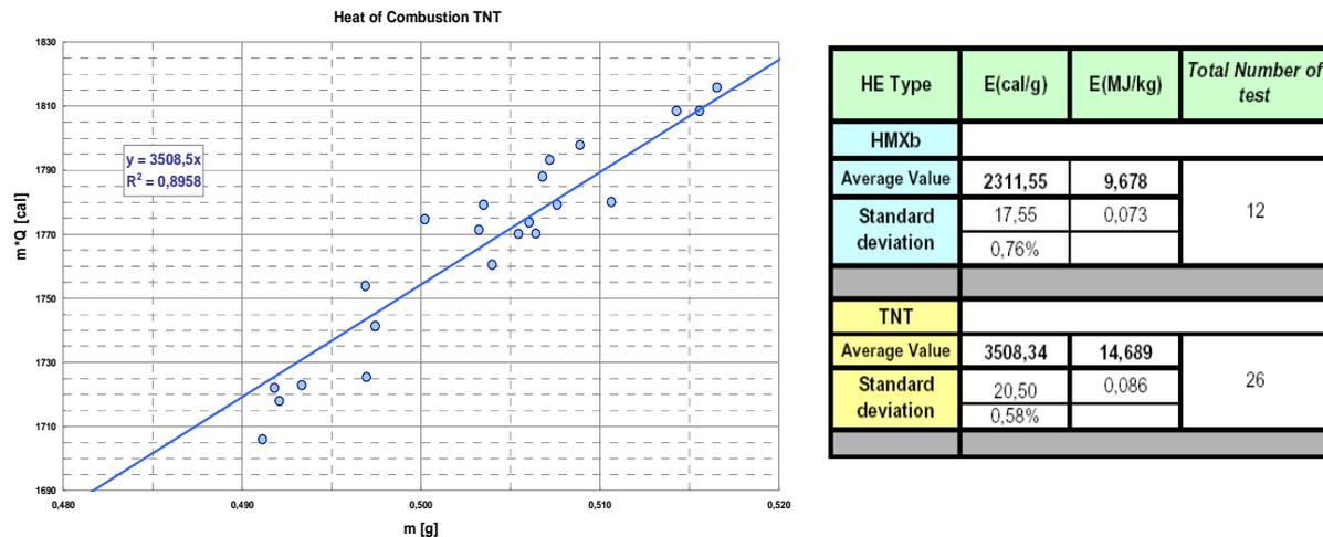
Figure 1 Left: Measured heat released in calorimetric bomb during TNT combustion under pure oxygen atmosphere as a function of the sample mass – Right: experimental values of combustion energy
