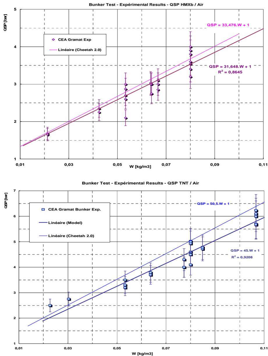
Figure 6 QSP Experimental results (absolute pressure) – Comparison with Cheetah calculations
