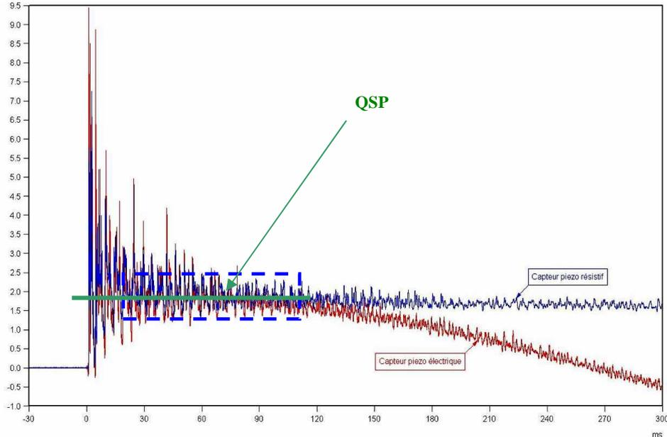
Figure 4 Typical signals: Overpressure time histories and QSP plateau (blue curve : piezoresistive transducer – red curve : piezoelectric transducer) – In blue, selected window to perform FFT
