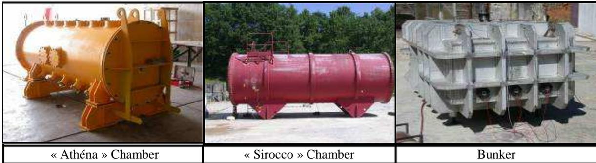
Figure 3 CEA Gramat hermetically sealed vessel dedicated to closed volume explosion
