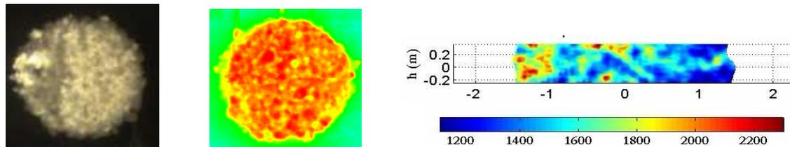
Figure 2 Fireball dynamics – Visualization of turbulent combustion (visible spectrum (left), pseudo color analysis (center) and surface temperature (right) in Kelvin (infrared pyrometer) for TNT (6 kg spherical charge)
