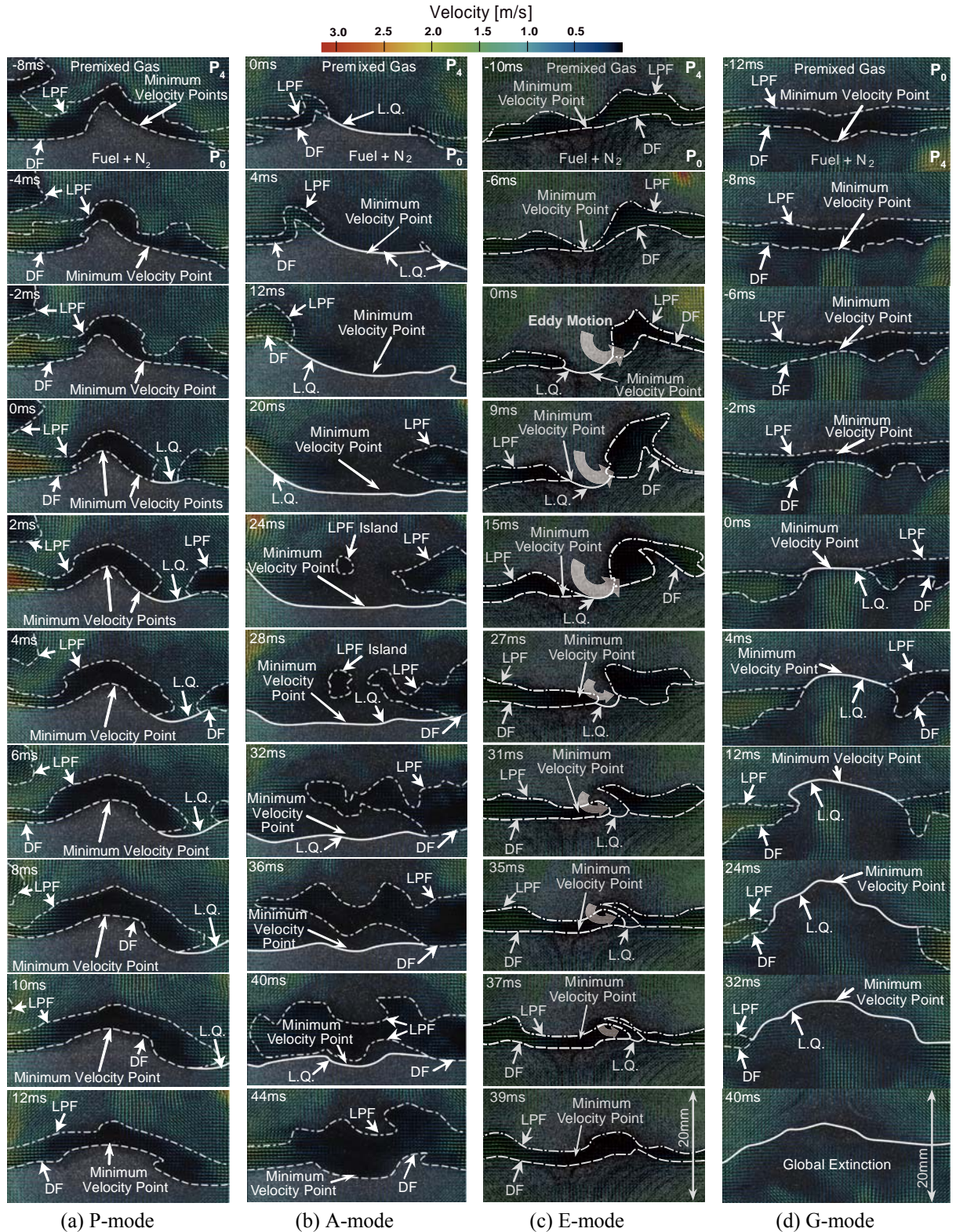
Figures 3. Four different local quenching modes. P-mode, A-mode, E-mode and G-mode correspond as passive local quenching recovery mode, active local quenching recovery mode, eddy transport local quenching recovery mode, and local quenching develops to global extinction, respectively. The flow conditions are following: (a) and (b) P_4/P_0 , \phi_U=0.6 , \chi_L=7.8\% ; (c) P_4/P_0 , \phi_U=0.3 , \chi_L=22.0\% ; (d) P_0/P_4 , \phi_U=0.6 , \chi_L=10.0\% .
