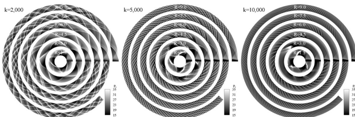
Figure 1. Smoked-foil records for different radii of curvature with different pre-exponential factor,  $k$ .
