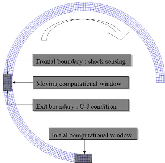
Figure 1 Grid system & Computational domain
