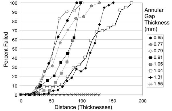
Figure 4: Analysis of rods showing percent of front failure as a function of propagation distance for aluminum confinement
