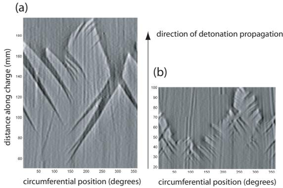
Figure 3: Laser scans of central rods for (a) 1.31 mm gap thickness and (b) 0.77 mm gap thickness. The dark regions indicate where detonation has failed.
