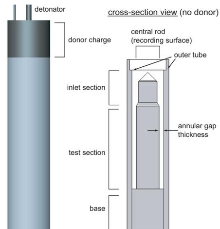
Figure 2: Charge design for annular experiment with central rod
