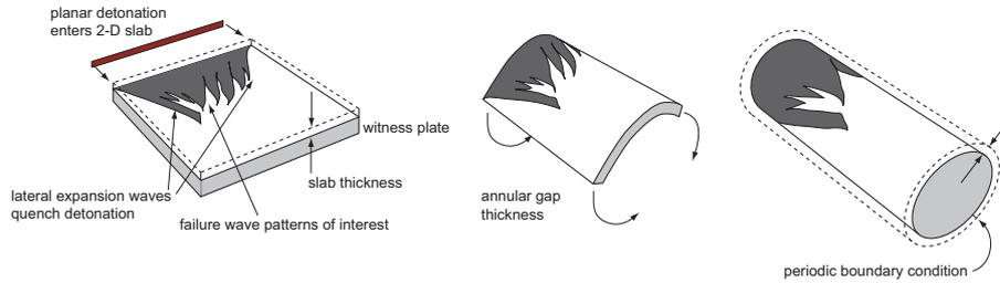
Figure 1: Schematic of an annular charge with periodic boundary conditions
