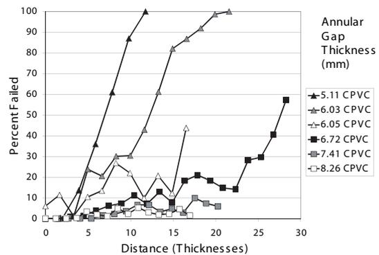
Figure 5: Analysis of rods showing percent of front failure as a function of propagation distance for PVC confinement
