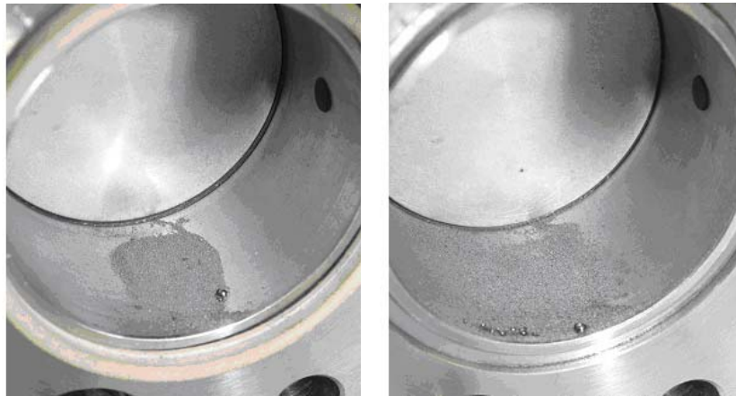
Figure 3. Photographs of test chamber with particle sample after compression for near critical conditions
