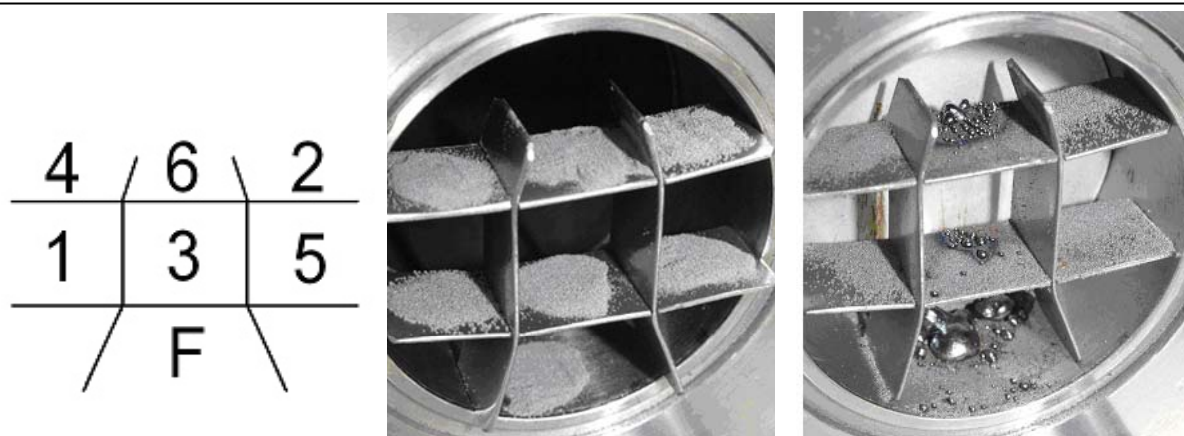
Figure 4. Plan of the fraction location on the rack shelves (left) and photographs of test chamber before and after compression .
