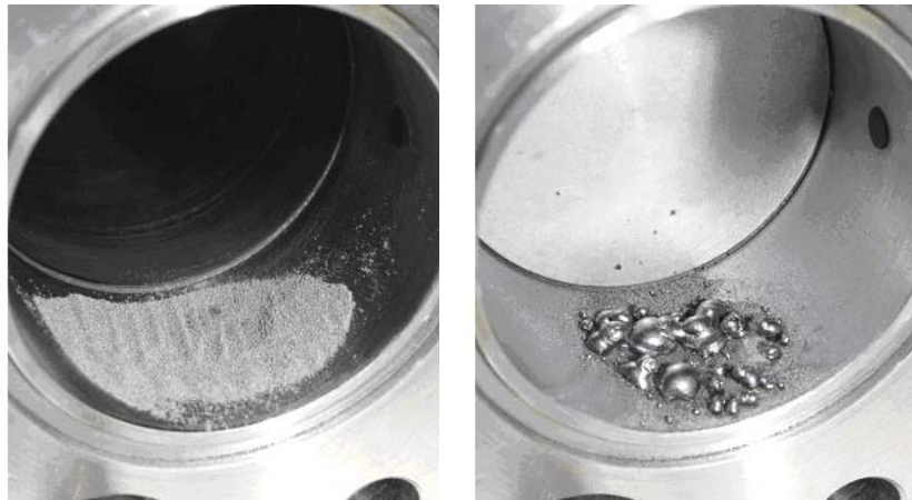
Figure 2. Photographs of test chamber with particle sample before (left) and after compression (right)
