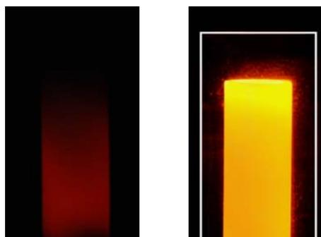
Figure 2. Photograph of combustion chamber operated without and with reverse tube.
