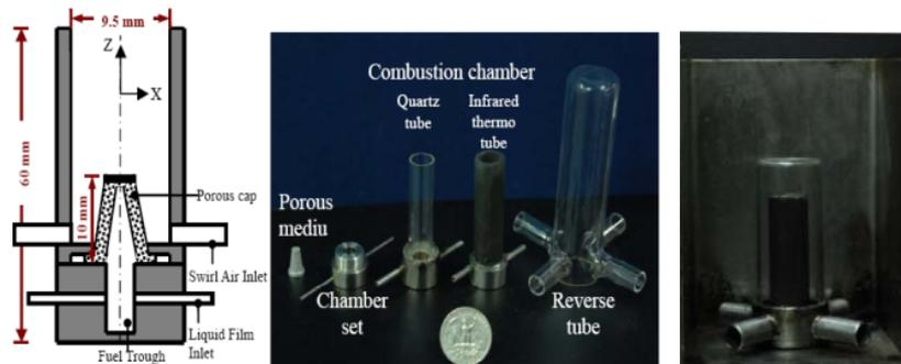
Figure 1. Schematic and photograph of the experimental combustor
