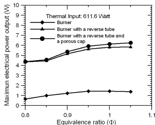
Figure 4. Electrical power output at different equivalence ratio
