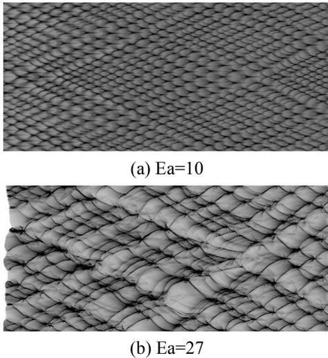
Figure 1. Trajectory of triple points in case of (a)  $E_a=10$  and (b)  $E_a=27$  at two-dimensional detonation
