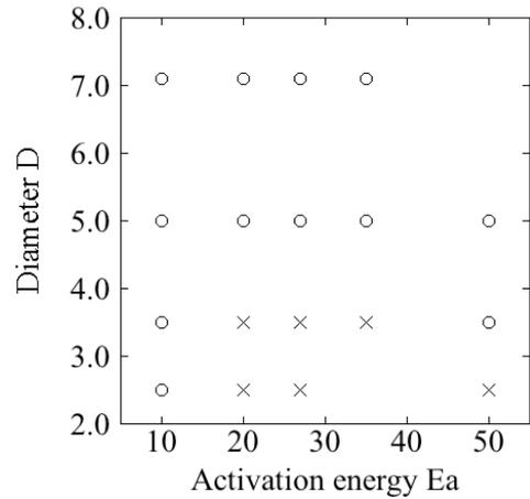
Figure 2. The propagation mode of spinning detonation as a function of activation energy and diameter.  $\circ$ : stable mode,  $\times$ : unstable mode
