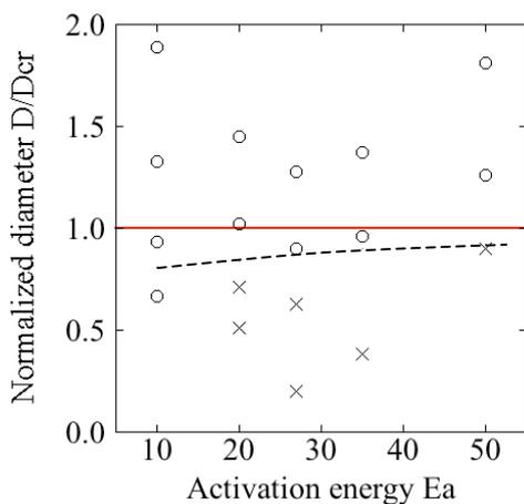
Figure 4. The propagation mode of spinning detonation as a function of activation energy and normalized diameter.  $\circ$ : stable mode,  $\times$ : unstable mode. Solid and dashed lines denotes  $D/D_{cr}=1$  and  $D/D_{cr}=\tan\alpha$ , respectively.
