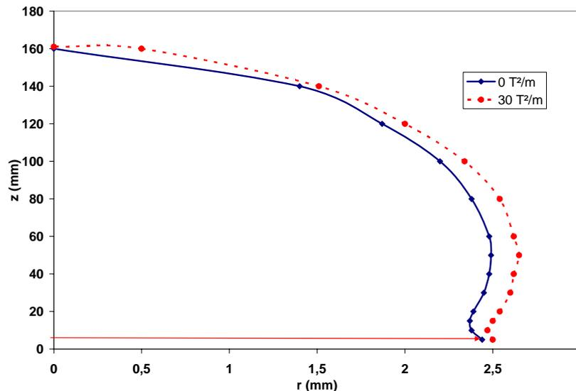
Figure 5:  $(r,z)$  evolution of the stoichiometric radius for the methane air laminar flame. (Red arrow corresponds to the vertical location of the maximum negative magnetic gradient)
