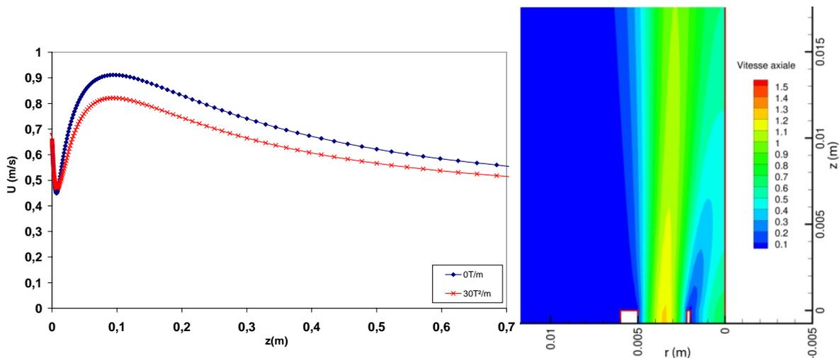
Figure 4: Velocity vertical component on z-axis. (Legend: blue=without magnetic force, red = with magnetic force)
