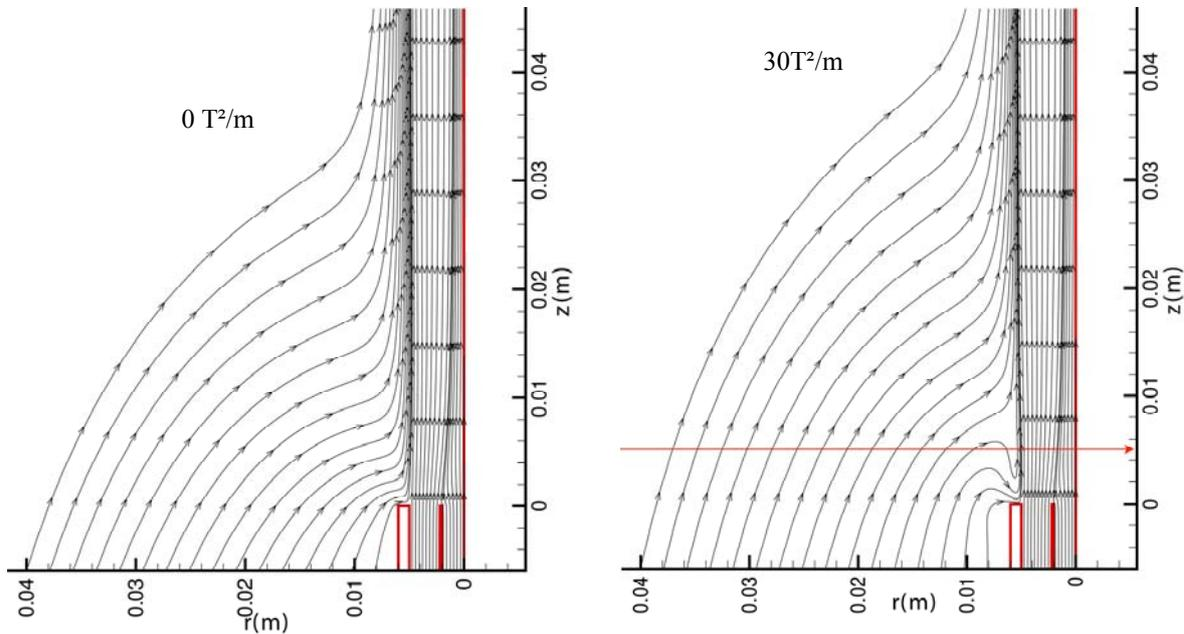
Figure 3: Streamlines of the jet flows without (left) and with the magnetic force (right). (Red arrow corresponds to the vertical location of the maximum negative magnetic gradient)
