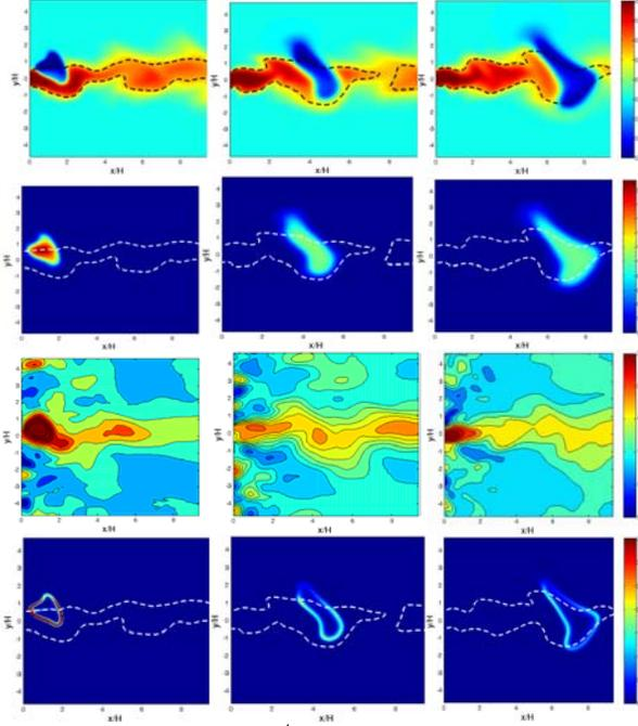
Figure 1. The fields of fuel mass fraction  $Y_F$  (1<sup>st</sup> row), non-dimensional temperature  $T$  (2<sup>nd</sup> row), axial velocity  $u_1$  (3<sup>rd</sup> row) and fuel reaction rate magnitude  $\dot{w}_F$  (4<sup>th</sup> row) at times  $t=1.00t_{sp}$  (1<sup>st</sup> column),  $t=4.20t_{sp}$  (2<sup>nd</sup> column) and  $t=7.40t_{sp}$  (3<sup>rd</sup> column). The  $\xi = \xi_{st}$  isosurface is shown by black (white) broken lines on the  $Y_F$  ( $T$  and  $\dot{w}_F$ ) fields.
