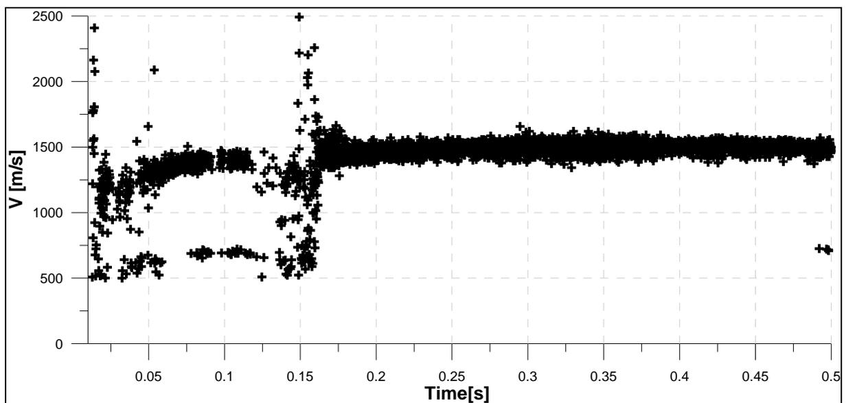
**Figure 4.** Detonation velocity-time history evaluated from recorded peak pressures on the outer chamber wall for methane-oxygen mixture; initial pressure was 0,1bar (small chamber with aerospike nozzle).
