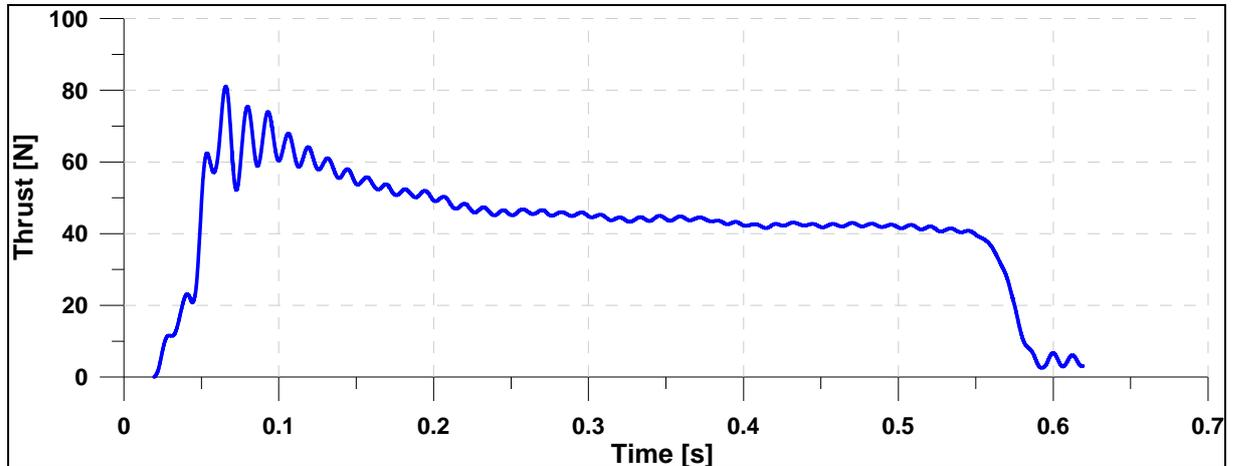
**Figure 5.** Thrust-time profile for methane-oxygen mixture, initial pressure was 0,1bar (small chamber with aerospike nozzle).
