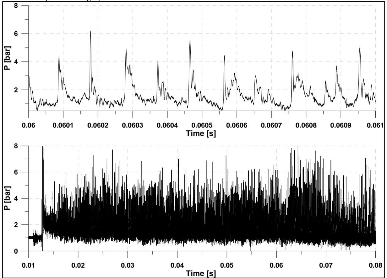
**Figure 3.** Pressure-time history recorded on the outer chamber wall for methane-oxygen mixture, initial pressure was 1bar (small chamber, cylindrical shape of the wall).
