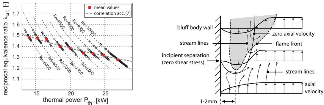
Figure 3: Stability limits of the investigated swirl burner for  $CH_4$ -air mixture.
