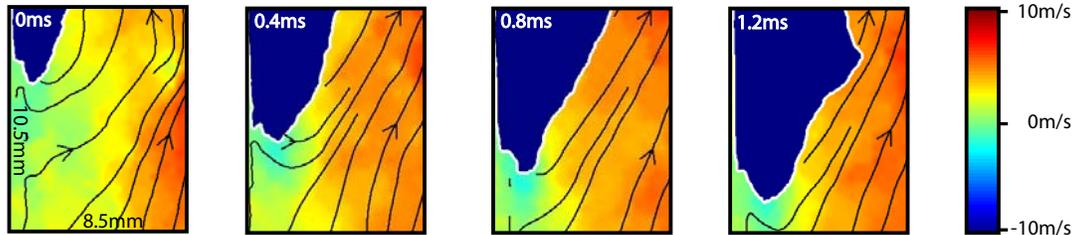
Figure 5: Sequence of leading edge upstream propagation from PIV data. Dark blue area: hot exhaust gas, background colours: axial velocity, lines: streamlines.
