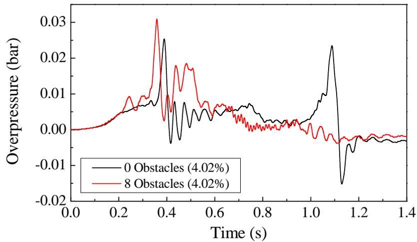
Figure 3. Effect of obstacles for stoichiometric propane-air mixtures with center ignition and a 5.43 m<sup>2</sup> vent.
