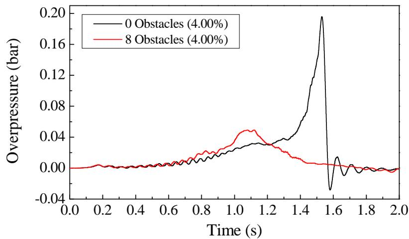
Figure 4. Effect of obstacles for stoichiometric propane-air mixtures with front-wall ignition and a 2.73 m<sup>2</sup> vent.
