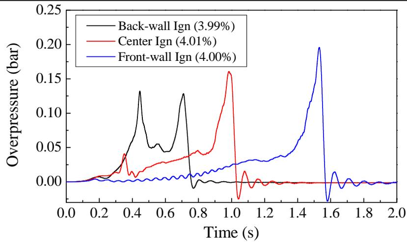
Figure 2. Effect of ignition location for stoichiometric propane-air mixtures with 0 obstacles with a 2.73 m<sup>2</sup> vent.
