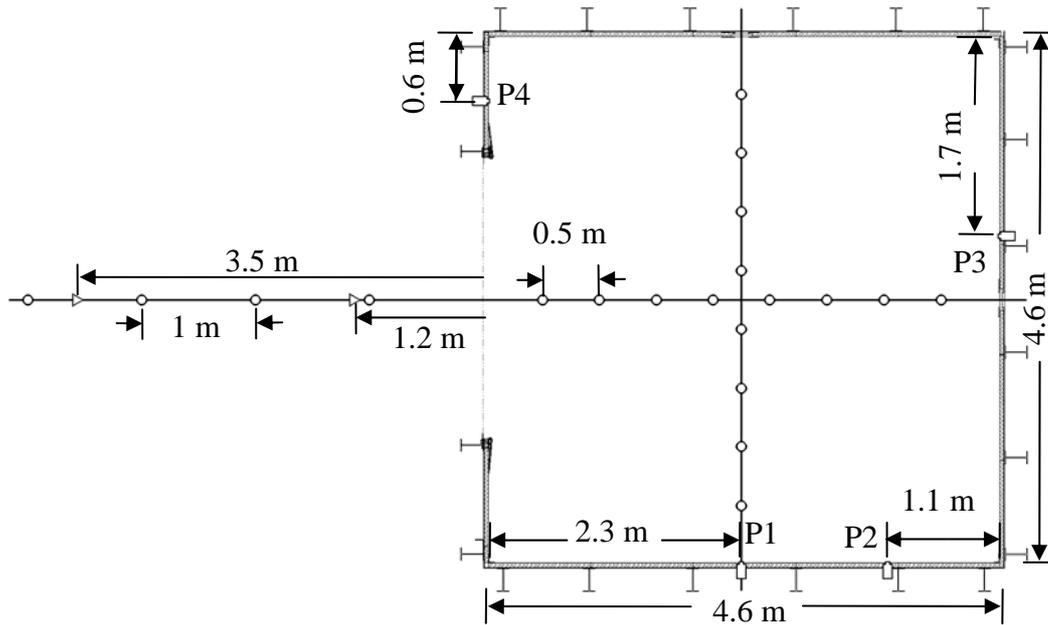
Figure 1. Illustration showing the locations of pressure transducers, (rectangles), flame arrival thermocouples (circles), blast-wave pressure transducers (triangles).
