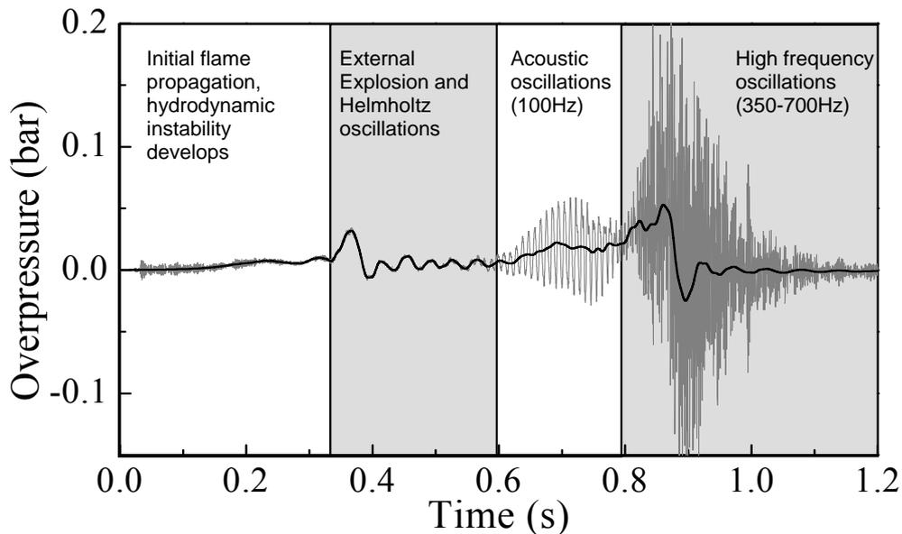
Figure 1. Filtered and unfiltered pressure time history of a stoichiometric propane-air mixture used to illustrate major phenomena observed during a typical vent explosion test.
