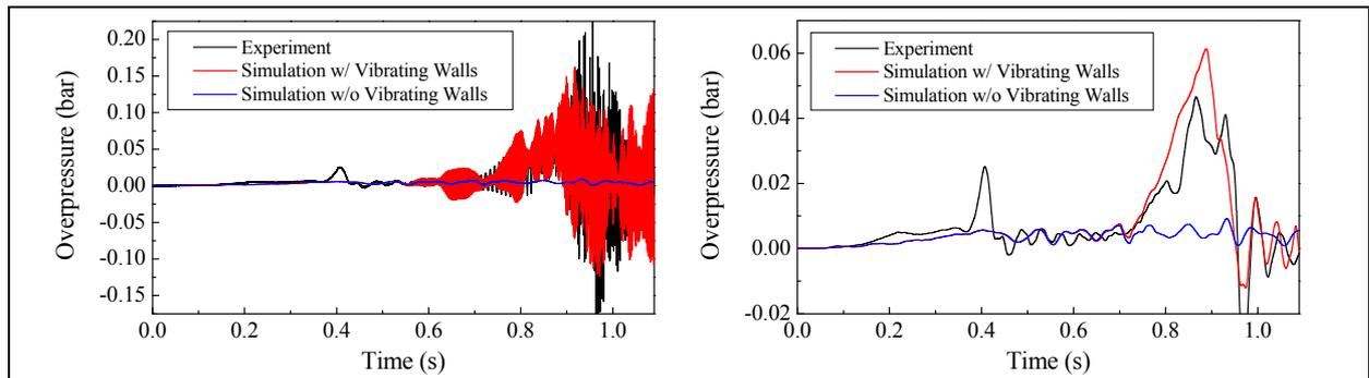
Figure 3. Comparison between experiments and simulations of a vented explosion, with unfiltered results on the left, and filtered by an 80 Hz low pass filter on the right.
