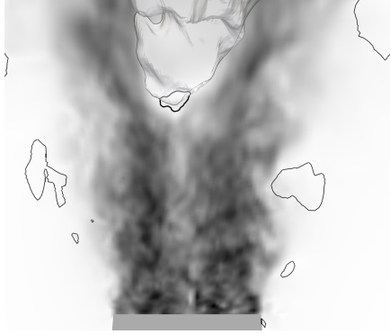
Figure 3: Snapshot during a CIVB flashback. Contours of velocity magnitude, recirculation zone marked with an isoline of zero axial velocity and flame front marked by the surface of \tilde{c} = 0.5 .
