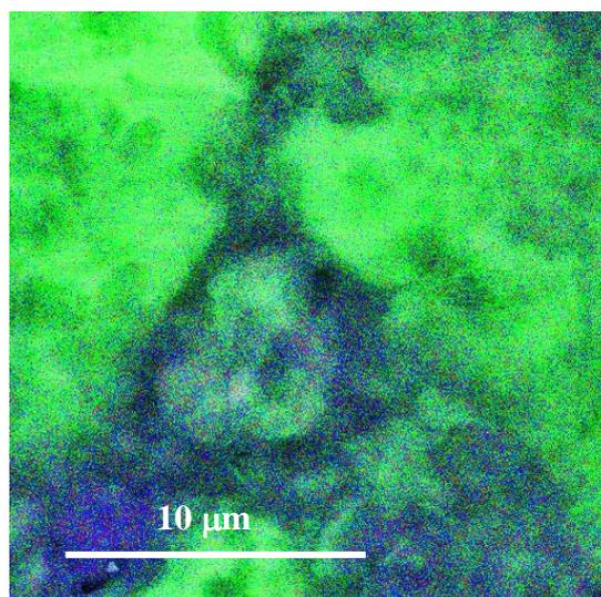
Figure 2. SEM image of the as-prepared SiO<sub>2</sub>/Al mechanocomposite. Green and blue colors indicate Al and Si, respectively.
