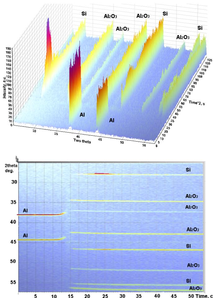
Figure 3. Kinetics of the phase transformation of the SiO<sub>2</sub>/Al mechanocomposite during the SHS process followed by the time-resolved diffraction (top). Projection of the XRD patterns on the angle-time plane (bottom).
