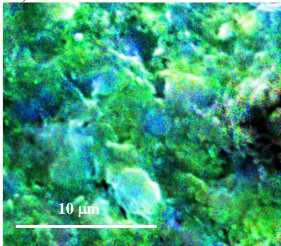
Figure 4. SEM image of the product (Si/Al<sub>2</sub>O<sub>3</sub> composite) of the SHS process. Green and blue colors indicate Al and Si, respectively
