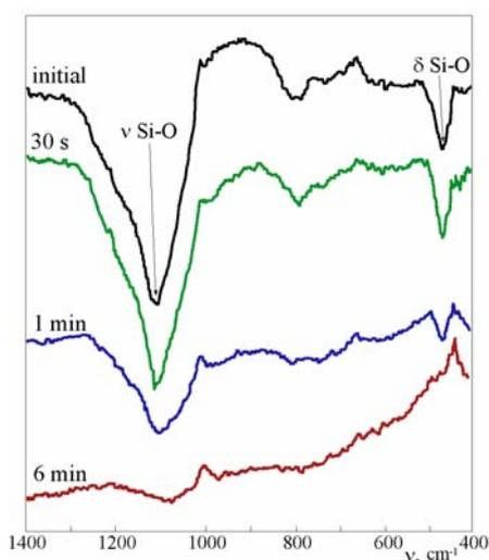
Figure 1. IR spectra of the SiO<sub>2</sub>/Al mixture mechanically activated for various times. The milling times are shown in the figure.
