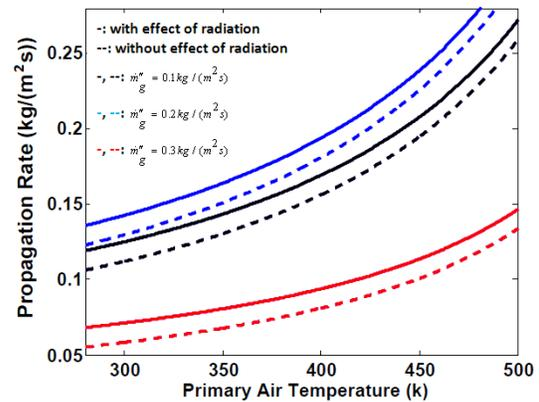
Fig. 2. Effect of primary air temperature on the propagation rate of the reaction front.
