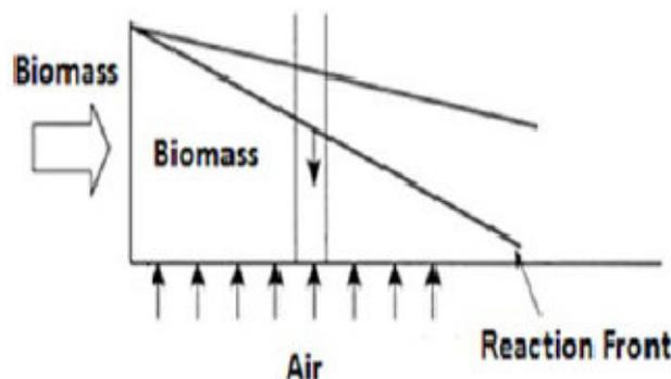
Fig 1. Schematic view of the combustion in bed of solid fuel
