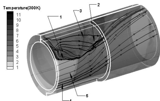
**Fig. 5** Temperature distribution at  $72 \mu\text{s}$ . 1-detonation wave, 2-oblique shock wave, 3-slip line, 4-triangle zone of fresh premixed gas, 5-stream lines
