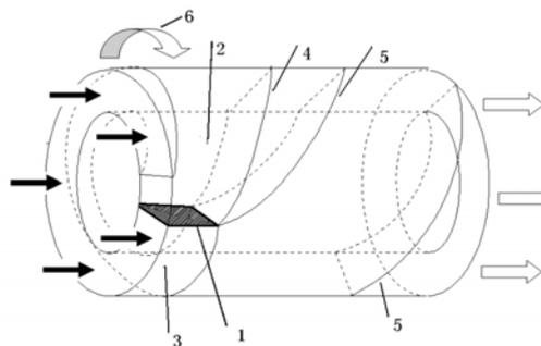
**Fig. 1** RDE propagation schematic structure. 1-detonation wave, 2-burnt product, 3-fresh premixed gas, 4-slip line, 5-oblique shock wave, 6-detonation wave propagation direction.
