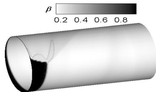
**Fig. 2** Chemical reaction process parameter  $\beta$  distribution in two-dimensional simulations.  $\beta=1$  means fresh fuel,  $\beta=0$  mean completely combusted product.
