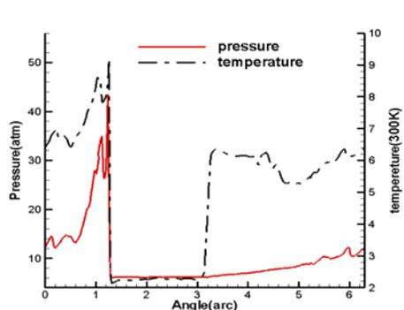
**Fig. 7** Pressure and temperature distribution along a circle line at position  $r=1.15\text{cm}$ ,  $z=0.2\text{cm}$  at  $72 \mu\text{s}$ .
