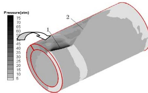
**Fig. 4** Pressure distribution at 72  $\mu$ s .1-detonation wave, 2-oblique shock wave. The arrow indicates the detonation wave propagate direction.
