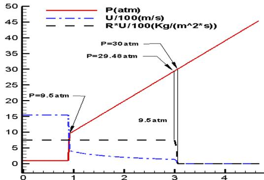
**Fig. 3** Relationship between wall pressure, inject velocity and mass flux of injecting mixture.
