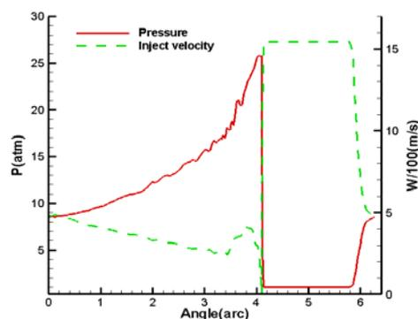
**Fig. 8** Pressure and inject velocity distribution just near the head wall along a circle line which is at  $r=1.15\text{cm}$ ,  $z=0$  at  $87 \mu\text{s}$ .
