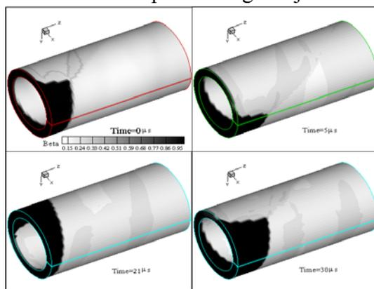
Fig. 10 Reaction progress parameter  $\beta$  distribution in one cycle form 0-30  $\mu\text{s}$ .
