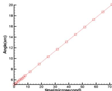
**Fig. 9** Detonation wave front position from  $0-72 \mu\text{s}$ .
