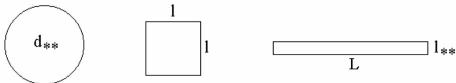
Fig.4. Schema of simplest transformation of charge symmetry: the round orifice of diameter  $d_{**}$  ensures the spherical initiation in a mixture volume, and a rectangular orifice with dimensions  $L \times l$  at  $L \gg l$  ensures the cylindrical initiation at  $l > l_{**}$ .
