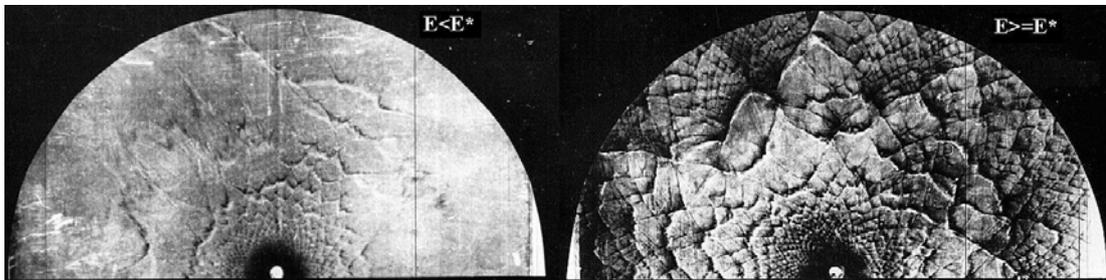
Fig.3. The smoked imprints of subcritical (left,  $E < E^*$ ) and critical (right,  $E \approx E^*$ ) DW initiation with the help of exploding wire.
