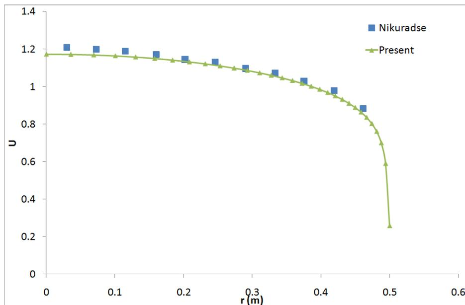
Figure 5: Velocity profile at the outlet of the pipe compared to those of Nikuradse's.
