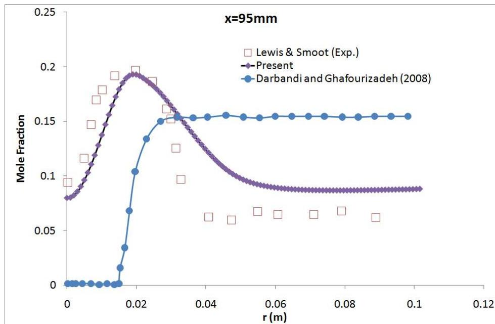
Figure 20: Radial distribution of the mole fraction compared to that of Darbandi and Ghafourizadeh [2] and experimental data [6].
