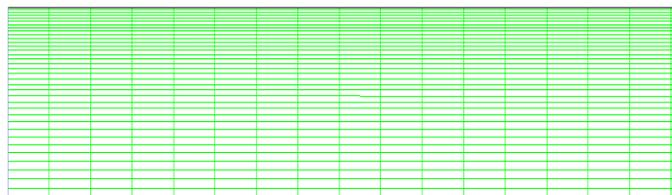
Figure 2: A portion of the grid used for the analysis of the non-reactive pipe flow.
