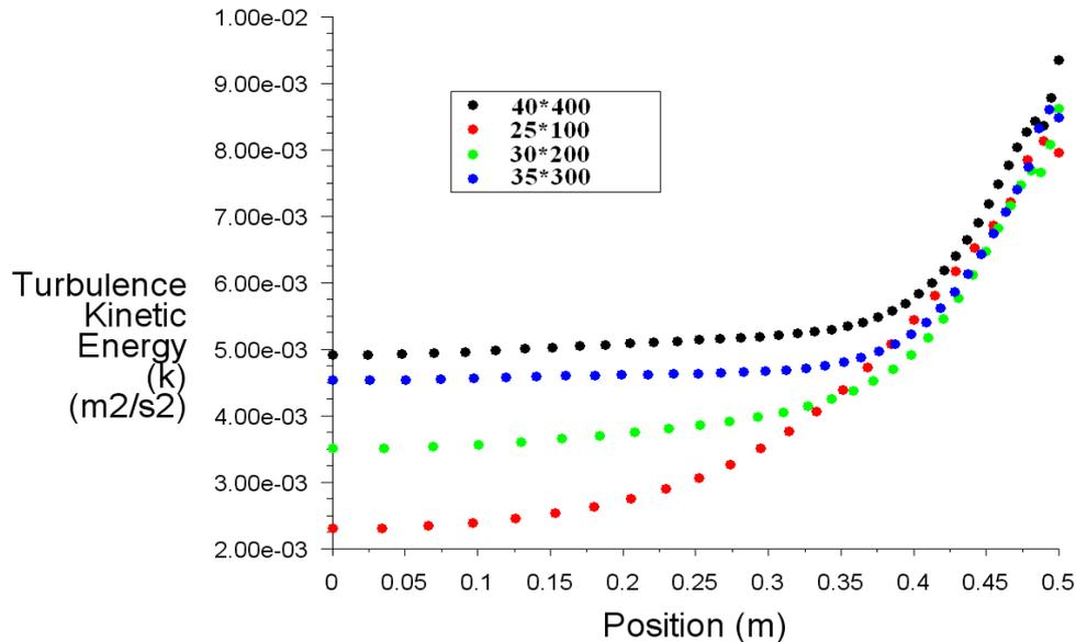
Figure 3: Radial distribution of the turbulence kinetic energy at the outlet of the pipe for 4 different mesh resolutions.
