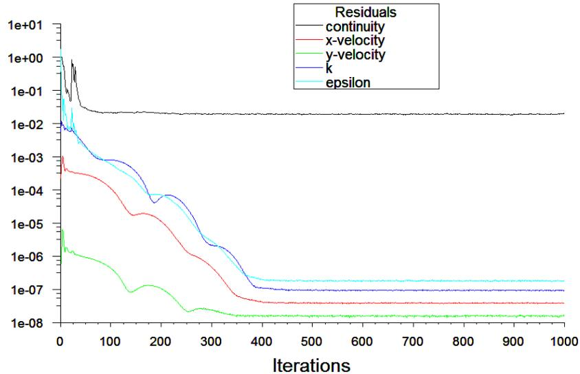
Figure 4: Residual history for the non-reactive pipe flow.
