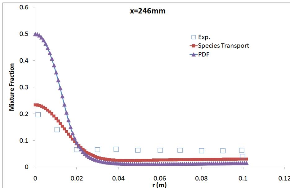
Figure 9: Radial distribution of the mixture fraction using the species transport and the PDF models.
