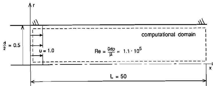
Figure 1: Geometrical and inflow properties of the non-reactive pipe flow.
