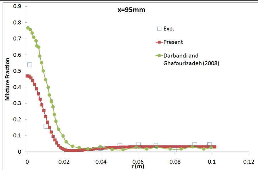
Figure 8: Radial distribution of the mixture fraction compared to that of Darbandi and Ghafourizadeh [2] and experimental data [6].
