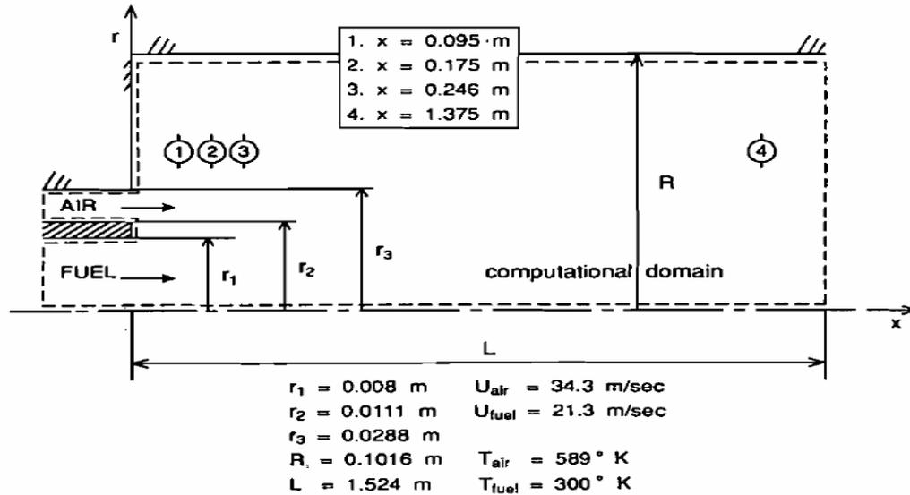
Figure 6: Geometrical and inflow properties of the reactive flow for the combustor.
