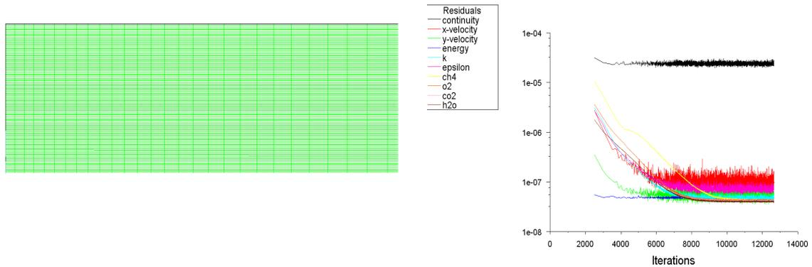
Figure 7: left: Grid used for the analysis, Right: residual history of the reactive flow inside a combustor.
