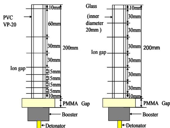
Fig.2 Assembly for electrical method
