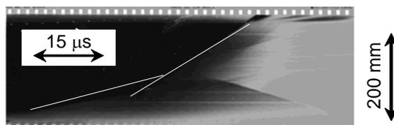
Fig.3 An example of a streak photograph (PVC tube, 15 mm gap)
