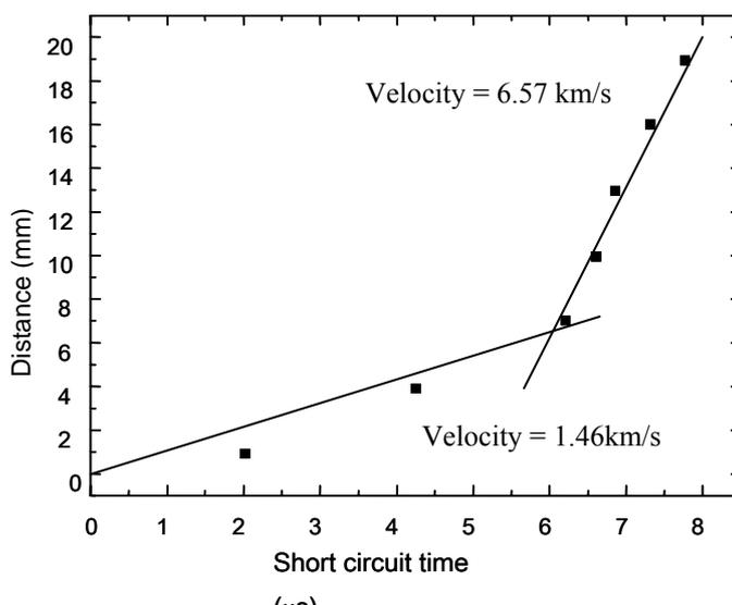
Fig.4 Relation of time and distance (glass tube, 15 mm gap)
