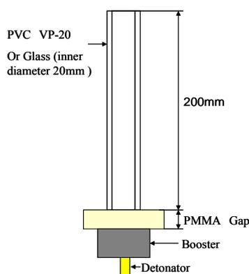
Fig.1 Assembly for optical method
