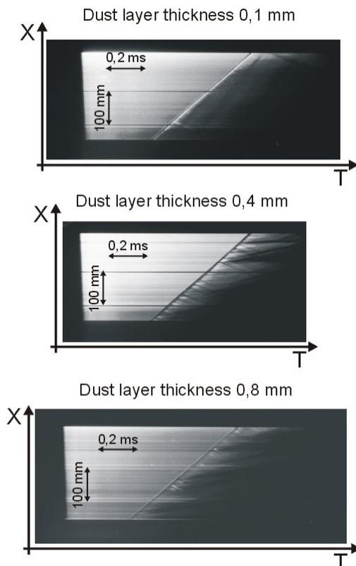
Fig. 6. Streak pictures of coal dust lifting.
