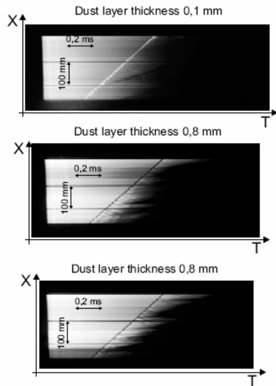
Fig. 7. Streak pictures of silicon dust lifting.
