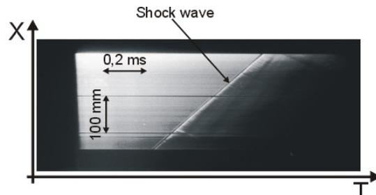
Fig. 5. Exemplary streak picture of the dust lifting up process: T – time, X – length of the slot
