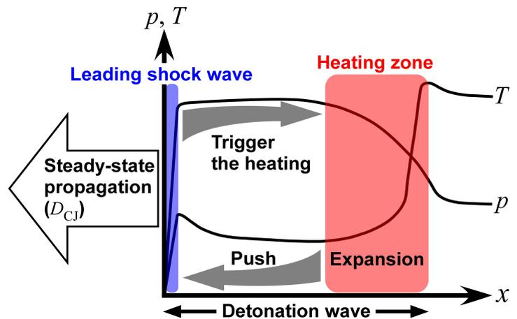
Fig. 1 One-dimensional model of a detonation wave.
