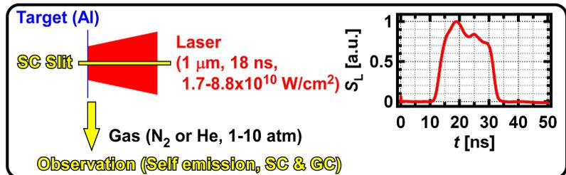
Fig. 2 Schematic of the experimental arrangement.
