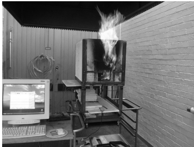
Fig.2.1 Picture of the experimental facility. Pool fire configuration.
