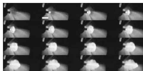
Figure 2 Images of development of the hydrogen-enriched plasma jet into the air environment. Exposure time of a film frame was 8 \mu\text{s} . A length of the line shown on second frame is 20 mm
