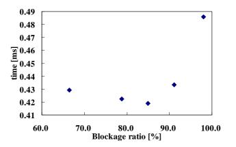
Figure 6 The blockage ratio vs DDT time for the mixture of 2H2 and O2.
