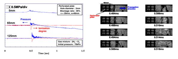
Figure 4 Pressure profiles using two perforated plates
