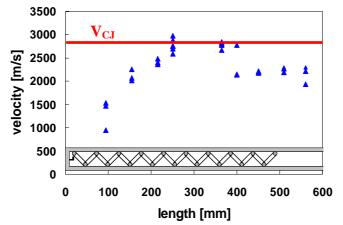
Figure 2 Propagation velocity using the Shchelkin wire for 2H<sub>2</sub>/O<sub>2</sub> cases.
