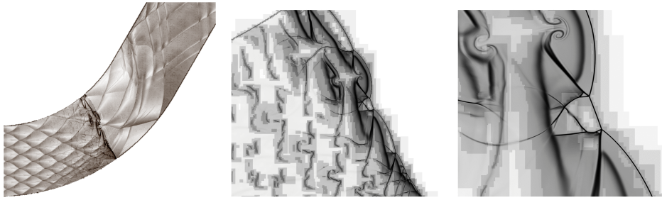
Figure 1: Schlieren plot of density on triple point tracks (left) and on refinement regions (shaded gray, middle and right) for \varphi = 45^\circ after t = 150 \mu\text{s} simulated time.
