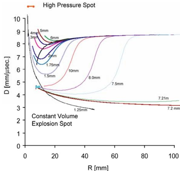
**Figure 1. The simulated  $D_n$ - $R$  response for PBX-9501, initiated from various hot-spot radii, both spherical low pressure and high pressure**
