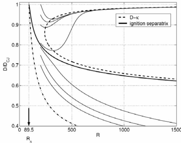
**Figure 2. Solution to equation (2), from reference [7] for a model of stoichiometric hydrogen-oxygen. The dashed dot line to the left is the D-R curve from the reactive blast wave solution that defines a critical energy and radius.**
