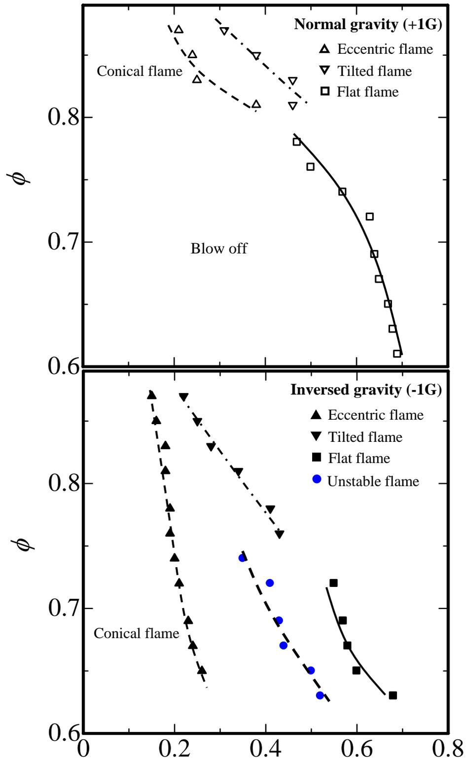
Figure 3: Stability map of flame shapes with burner rotation  $S$  as functions of equivalence ratio  $\phi$  and swirl number  $S$  for a constant axial flow velocity of  $U = 1.0$  m/s in normal gravity (+1G) and Inversed gravity (-1G)
