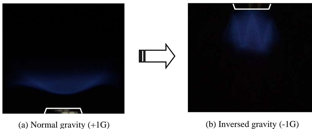
Figure 2: Flame shape of rotating flames under condition of  $U = 1.0$  m/s,  $\phi = 0.75$ ,  $S = 0.6$  in normal gravity (+1G) and inversed gravity (-1G)
