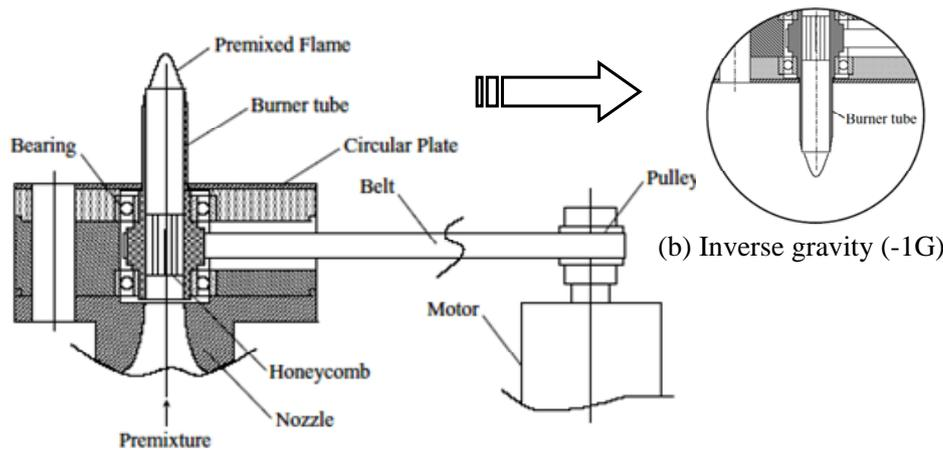
Figure 1: Experimental apparatus ((a) Normal gravity (+1G))
