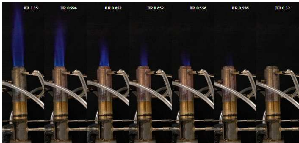
Fig 1: Effect of secondary air injection changing the air flow from 135 mg/s (equivalence ratio, ER 1.35) to 570 mg/s (ER 0.32) in different distributions of air injection between mid and top injectors.
