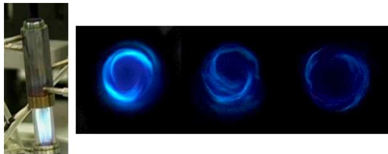
Fig 2 : Tubular flame images from side view through a sapphire window and from a top view with exposure time respectively (from left to right) of 0.001s, 0.00025s and 0.000125s .
