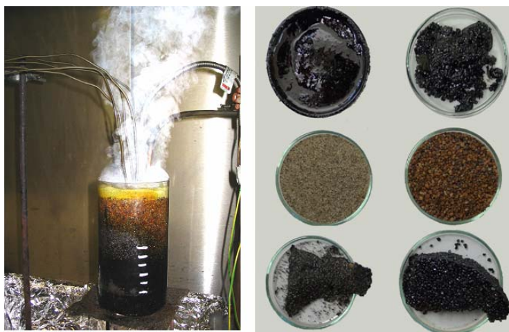
Figure 1. (Left): . (Right top) Fine and coarse sands contaminated with coal tar; (Right middle) remediated fine and coarse sands from within smouldering zone; and (Right bottom) resulting fine and coarse samples from outside smouldering zone.
