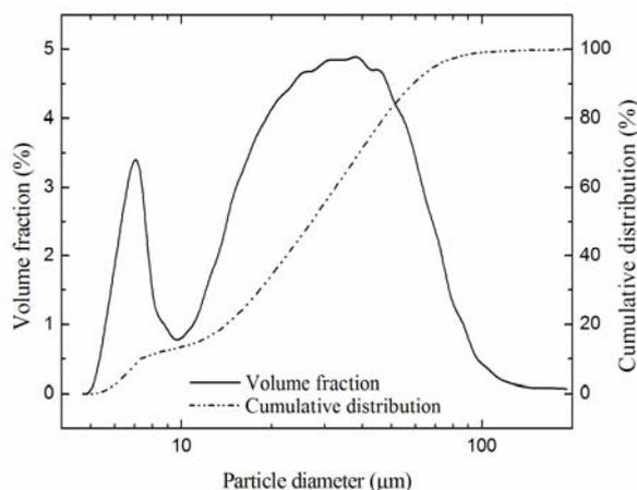
Fig.1b Size distribution of the raw material.
