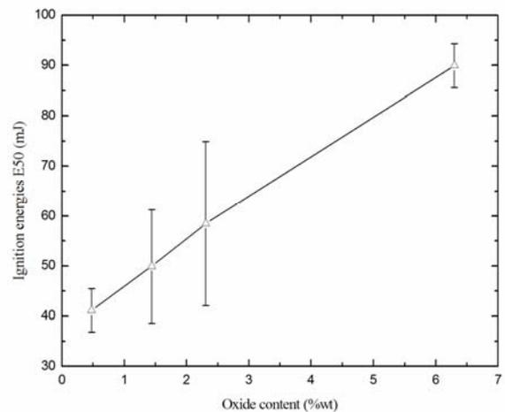
Fig.3 Influence of oxide content on ignition energies (equivalent ratio  $\sim 1$ ).
