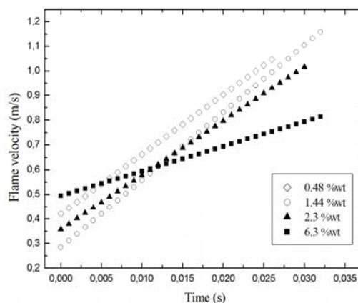
Fig.5b Influence of oxide content on flame velocity
