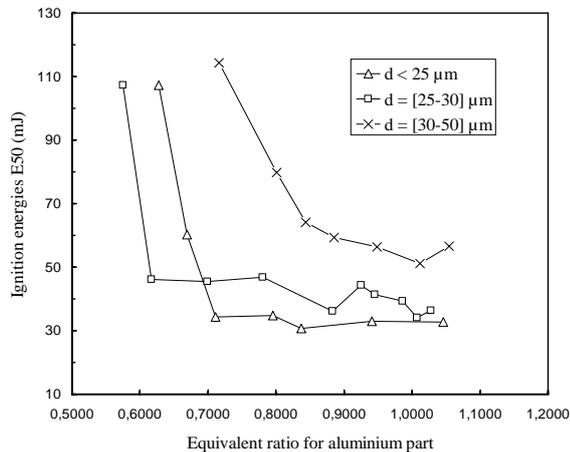
Fig.2 Influence of size distribution and dust concentration on ignition energies.
