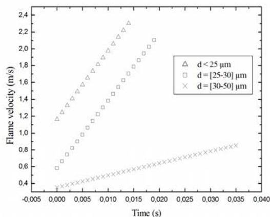
Fig.5a Influence of size distribution on flame velocity (t=0 at the end of ignition spark)
