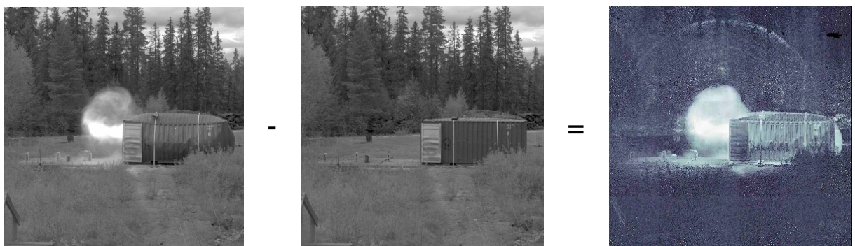
Figure 1. Principle of the image processing
