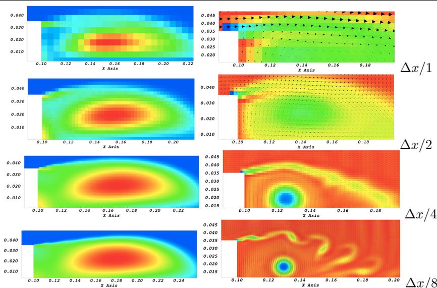
Figure 2: Unsteady flow over a backward facing step: plots of the integral length scale (left) and the vorticity on the filter scale (right) for different filter sizes  $\Delta x/n$  at a fixed time level, where  $\Delta x$  is the grid size of the coarsest grid. Grid is refined by a factor of two from top to bottom
