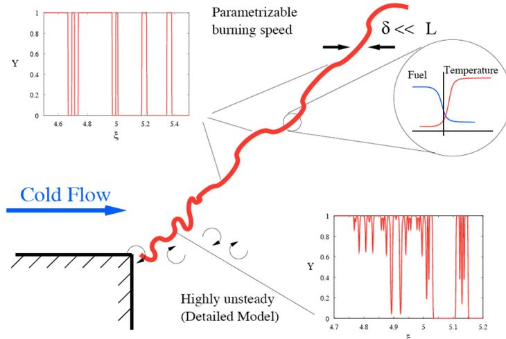
Figure 1: Flame attached to a flame holder: In highly unsteady regions a detailed flame structure computation, yielding the turbulent burning speed, is performed (lower right structure computed with LEM); if a parallel running parameterization yields comparable results, we switch off the costly online computation (upper left calculation, performed with LEM, switches to parameterization from eq. (1))
