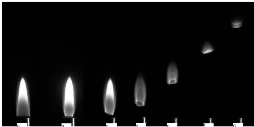
Figure 2: Flame configurations for a fixed methane velocity of .22m/s and increasing velocity of the air co-flow a)0, b).34, c).52, d).7, e).87, f)1.05, g)1.09 m/s
