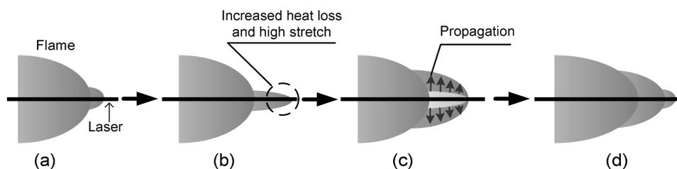
Fig.5 The hypothesis of flame oscillation mechanism
