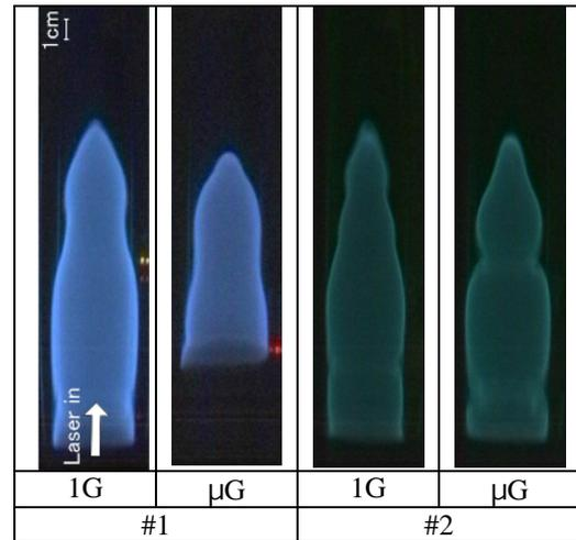
Fig.3 Still images of flame propagation with different gravity conditions (laser power 12W, FWHM 5mm)
