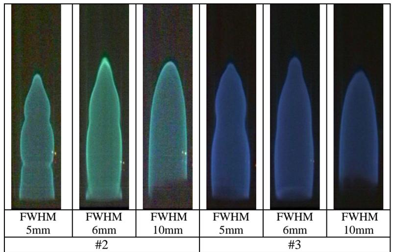
Fig.4 Still image of flame propagation with different Full-Width Half-Maximum (laser power 12W, normal gravity)
