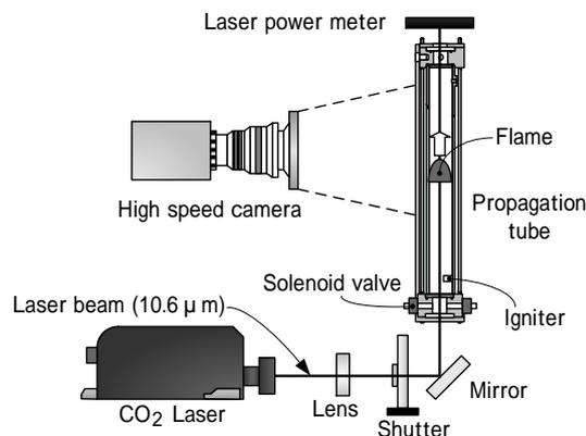
Fig.2 Schematics of experimental apparatus
