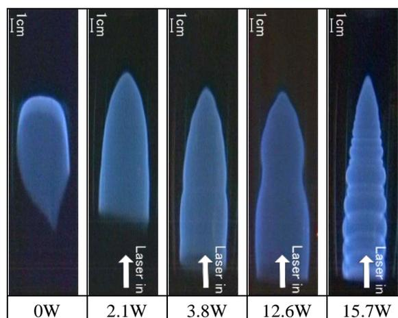
Fig.1 Still images of propagating ethylene-air premixed flames (tested gas is #3 ; see Table 1). with various applied laser powers in normal gravity condition. Propagating direction is from bottom to top. Laser is exposed from bottom (details are shown in Fig.2.)
