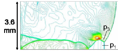
Fig. 2 Instantaneous pressure contours (post-shock pressures; p_1 , incident shock; p_3 , reflected shock).
