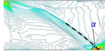
Fig. 3 Maximum pressure history ( \alpha , the entrance angle of the triple point track).
