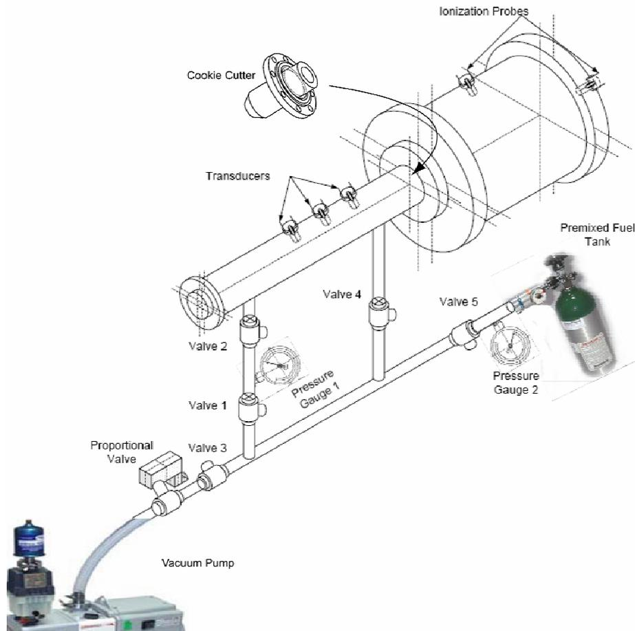
Figure 1: Schematic of apparatus for measurement of critical tube diameter.
