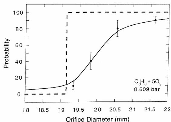
**Figure 3: Results from Fig. 2, shown as the probability of transition to unconfined detonation as a function to tube size, compared to the data (dashed) of Matsui and Lee [9].**
