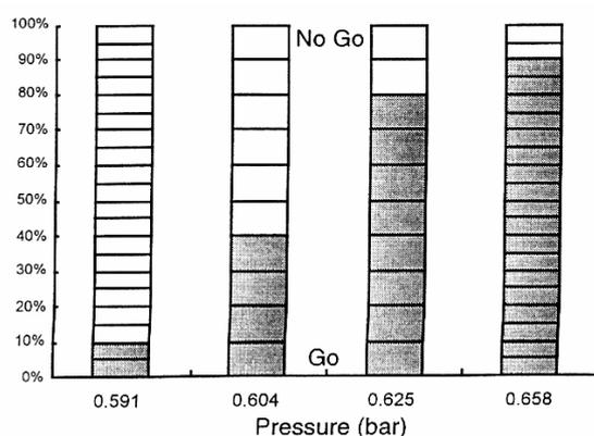
**Figure 2: Critical diameter results for  $C_3H_8+5O_2$  with 20 mm diameter tube, with open squares denoting “No Go” and shaded squared denoting “Go” results.**
